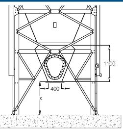
The 400mm  $\emptyset$  outlet suits Rotoflex Conveyors.
